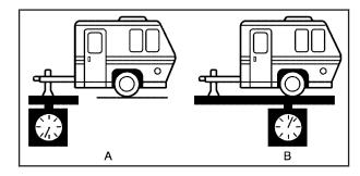
If you're using a weight-carrying hitch, the trailer tongue (A) should weigh 10 percent of the total loaded trailer weight (B). If you're using a weight-distributing hitch, the trailer tongue (A) should weigh 12 percent of the total loaded trailer weight (B).
